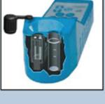
The pH/ORP sensor chamber provides protection to a unique porous liquidjunction.
